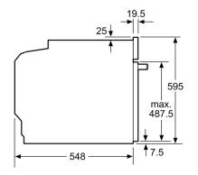
measurements in mm
